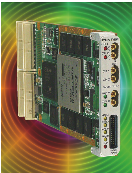
The Pentek Model 7140-420 dual digital transceiver features digital-downconverter and interpolation-filter intellectual-property cores to boost bandwidth range.
